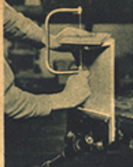
Using coping saw with saddle
