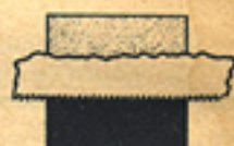
Fine teeth. No chip clearance. Teeth clogged
