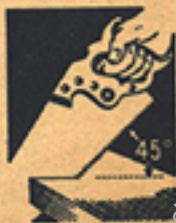
Proper angle for cross-cutting
