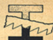
Coarse teeth straddles work stripping work
