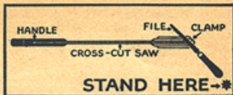
Second position for filing cross-cut saws
