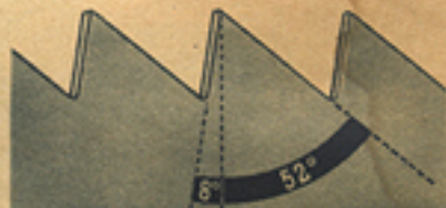
Side view of rip teeth (enlarged)
