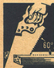
Proper angle for ripping
