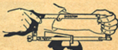
Proper way to hold hack saw frame when sawing
