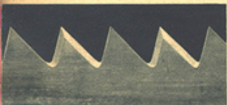
Shape of cross-cut saw teeth
