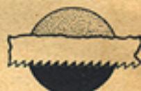
Fine teeth. No chip clearance. Teeth clogged
