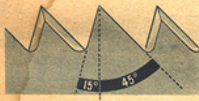
Side view of cross-cut teeth (enlarged)
