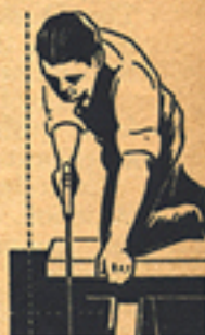
Proper position for cross-cutting
