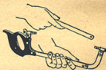
To insert blade in hack saw frame
